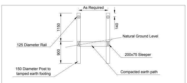
Posts to be installed at maximum of 2.4 centers. Sleepers cut to suit.
